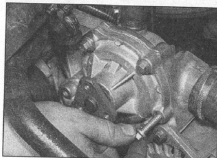
7.21 On 300 TDi engines, unscrew the retaining bolts . . .
